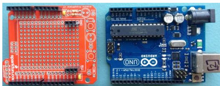
Figure 7 Arduino and Protoshield
