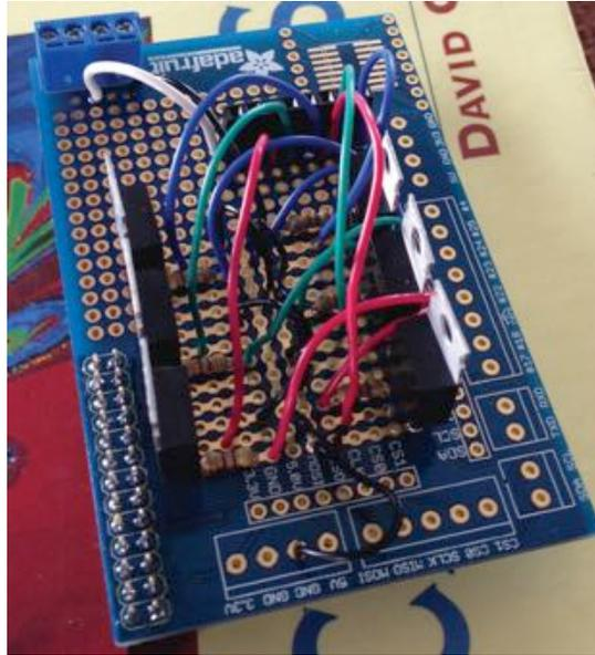
Figure 6 - LED driver board
