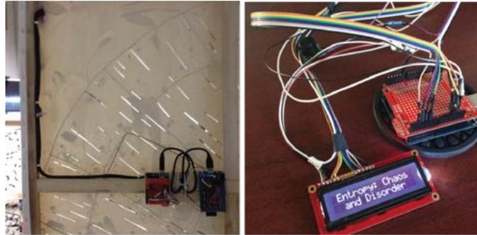
*Figure 8 – Left: SOTU computing hardware mounted to the frame. Wiring was secured in mesh cable management material and fastened to the frame using wire nails. Right: LCD screen displays the painting name “Entropy: Chaos and Disorder”*
