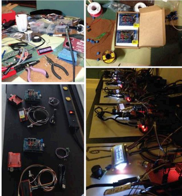
*Figure 17 - Top: Assembling and testing LCD screens and LED driver boards. Bottom: Assembling SOTU units and readying for functional test*
