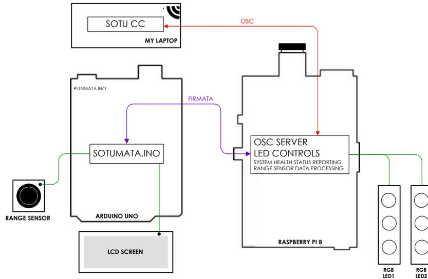
Figure 21 – Data flow during exhibition mode. Purple lines - Firmata messages over serial USB, green - GPIO output for LED activation and Analog output for range sensor readings, red - OSC.
