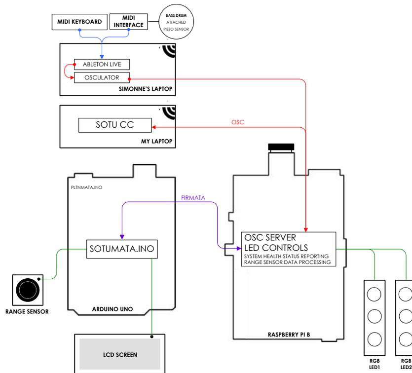
Figure 20 - OSC/MIDI message flow in performance mode. Blue lines represent MIDI, red, OSC, purple, Firmata, green, GPIO output for LED activation and Analog output for range sensor readings
