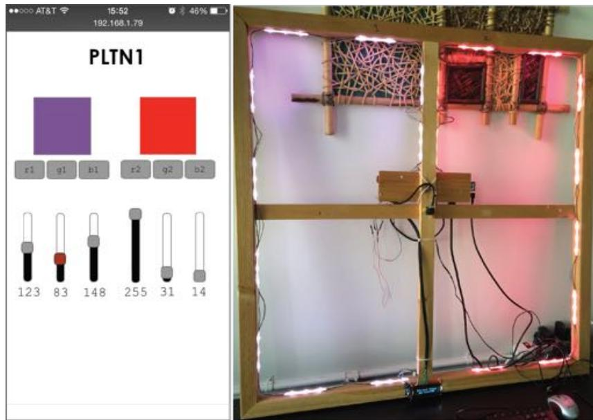
Figure 14 - Left: Web-based LED controller on an iPhone web browser. Right: lights change color based on web application
