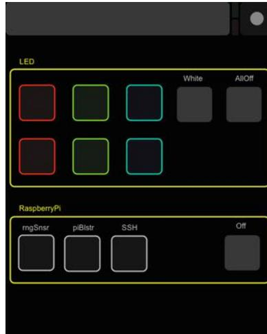
*Figure 13 - TouchOSC SOTU system testing UI. LED section of buttons controlled on/off associated colors for strip 1 and 2, turn all LEDs on/off to full white. Raspberry Pi section of buttons could turn the range sensor on/off, turn SSH or Pi-Blaster Linux services on/off, or turn the Pi itself off*
