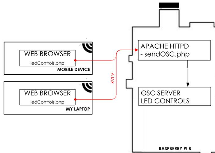
Figure 15 – Web LED application architecture. LEDs on each painting could be adjusted by accessing the ledControl.php web page individually served on each Raspberry Pi
